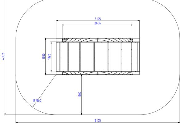
Fig. TERMA Inclusive spinning wheel dimensions with the safety zone
